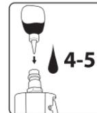
**NOTE:** Before the first use of the tool, apply 4-5 droplets of oil
