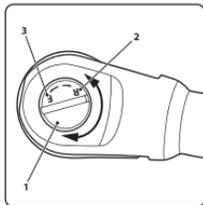
Check the set direction of rotation. To screw screws and nuts, set the switch in the F direction of rotation (Forward). To unscrew screws and nuts, set the switch in the R direction of rotation (Reverse). Check the position of the torque regulator: when unscrewing, the maximum torque is used; when screwing,
