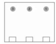
Figure 3-16: Pin Arrangement of RS485 interface
