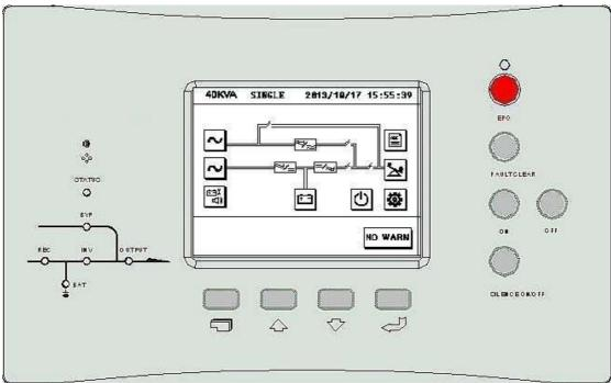
Figure 5-1: Operation Control and Display Panel of UPS
