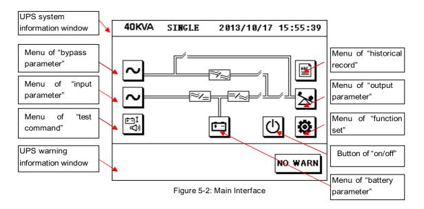
UPS system information window: to display basic information of UPS, including current time, date, UPS series name, configuration, and status. Information in this window cannot be operated by user, and detailed explanations are listed in Table 5-11:
