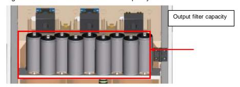
Figure 2-17: 60KVA UPS AC Output Capacity Module
