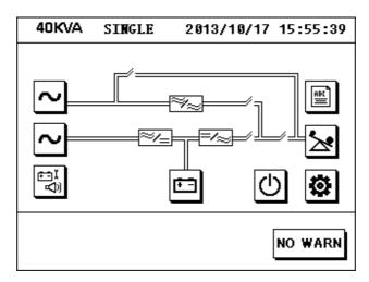
Figure 4-1: Power Flow Diagram after Normal Boot
