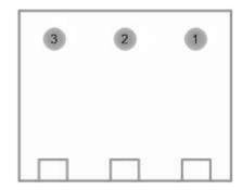
Figure 3-18: Pin Arrangement of Dry Contact OUT 1—8 Interface
