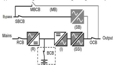
Figure 2-2: Main Power Supply Mode
