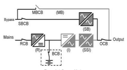
Figure 2-4: Bypass Mode
