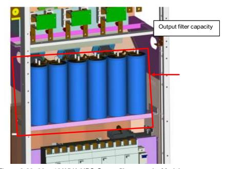
Figure 2-22: 80 ~ 120KVA UPS Output filter capacity Module
