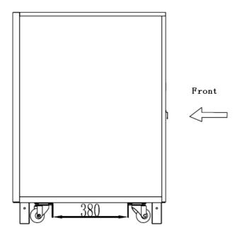
Figure 3-6: 10 ~ 40 KVA transport (Unit: mm)
