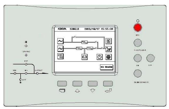
Figure 2-7: Liquid Crystal Panel
