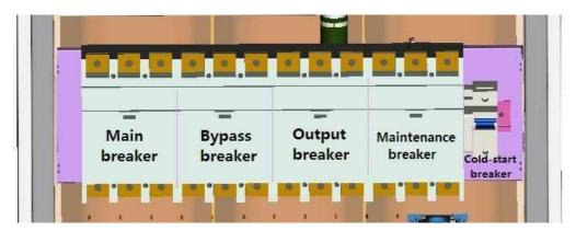
Figure 2-18: 60KVA UPS diagram of load switch
