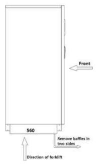
Figure 3-7: Carry of 60~120KVA (Unit: mm)
