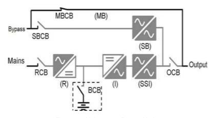
Figure 2-5: Maintenance Bypass Mode
