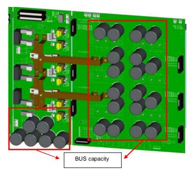
Figure 2-10: 10 ~ 40KVA BUS capacitance
